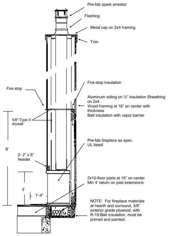
NOTE: Concrete wing wall or other approved support required on slab installations.
